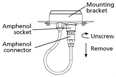
6. Connect the Extension cable to the Amphenol connector and tighten.
